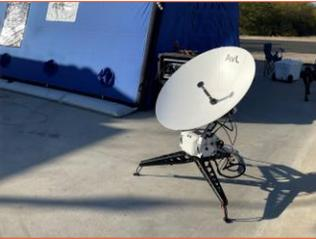
**Capabilities:** Provides satellite backhaul to macro sites when the standard backhaul is out of service.
